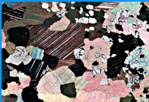
Fig.2 The carbonate 再結晶質石灰岩 Locality: Ibaraki pref. 茨城県柘山産 (cross-polarized light) (直交ニコル)
